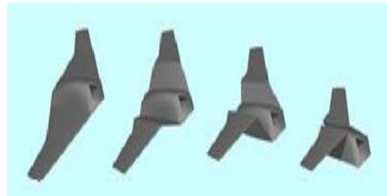
Fig. 5: “variable chord and variable sweep”
