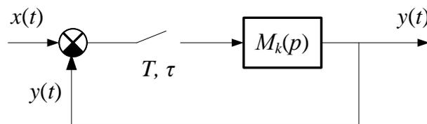
**Fig. 3.** Functional model of the system for analyzing transients
