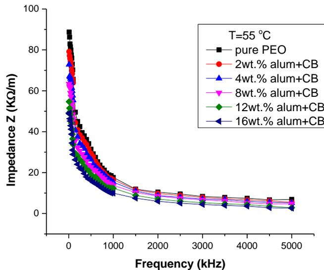
**Figure-3.** The variation of impedance with frequency for PEO/potassium aluminum sulfate samples
