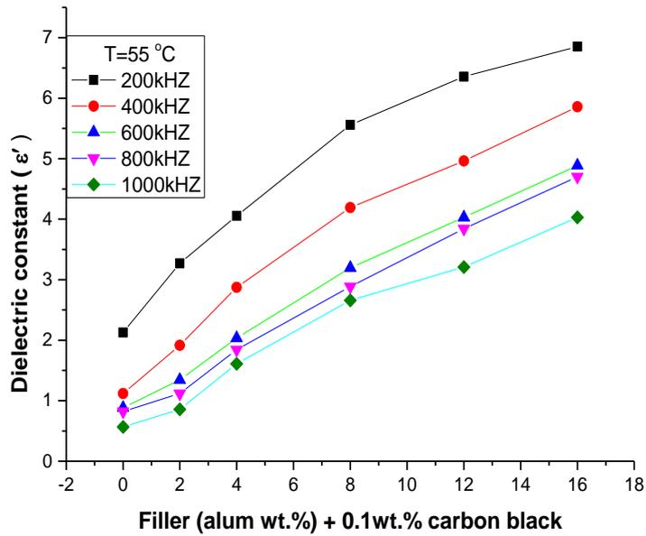
Figure-8. The dielectric constant versus potassium aluminum sulfate concentrations
