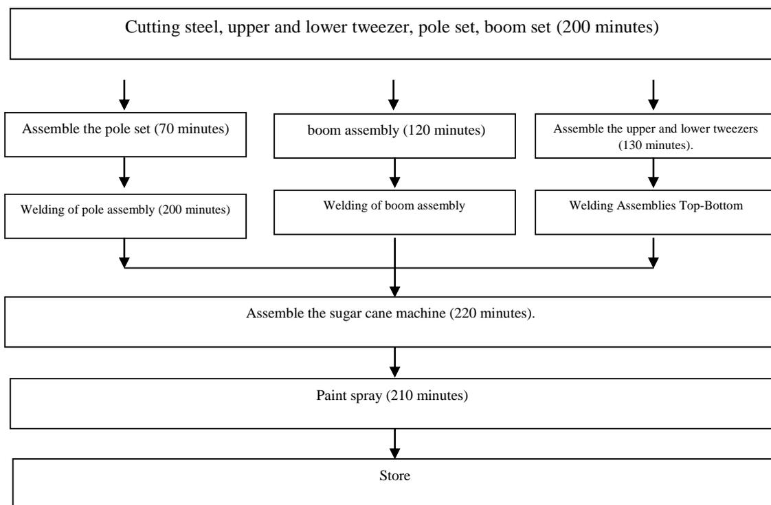
**Figure 2.** Production process of sugarcane grapple
