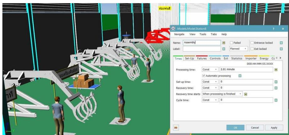
**Figure 8.** Calculation of capacity by computer program
