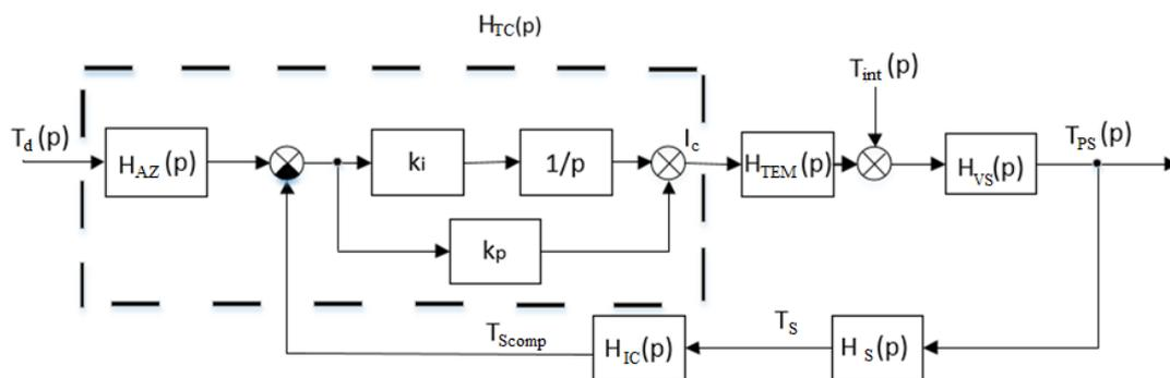
**Figure 3** - Equivalent functional model of the climate control system based on Peltier thermoelectric modules
