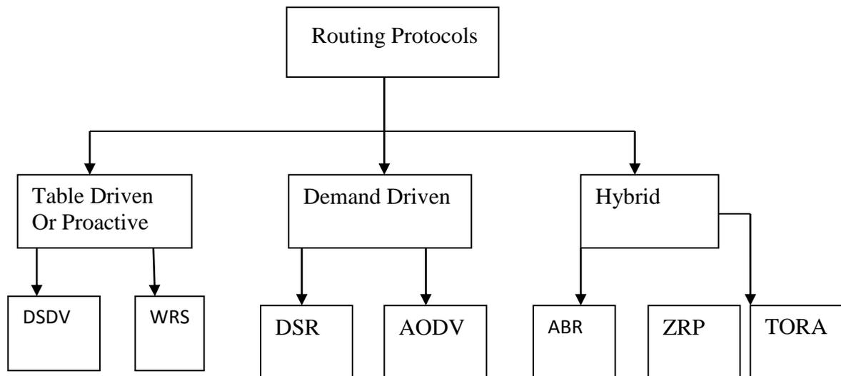
**Figure 1:** Classification of Routing Protocols
