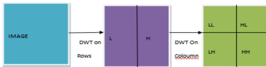
**Figure 16-** Block Diagram of DWT (a)Original Image (b) Output image after the 1-D applied on Row input (c) Output image after the second 1-D applied on row input
