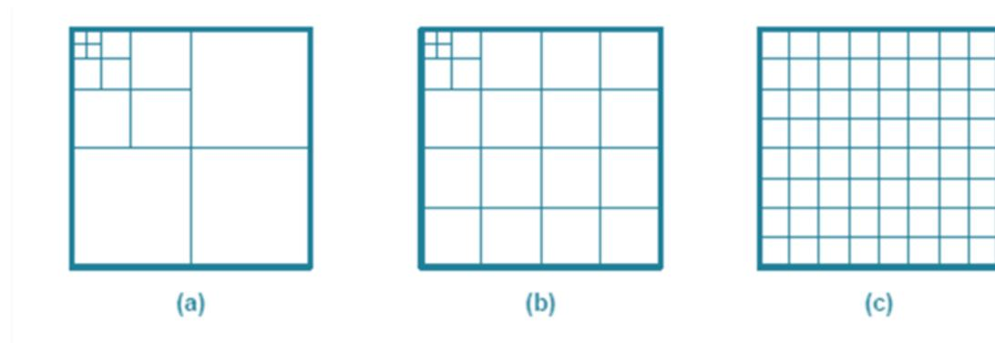
**Figure-9:** Three Popular Wavelet Decomposition Structures On Image: (a)Pyramid , (b) Spacl , (c) Wavelet packet
