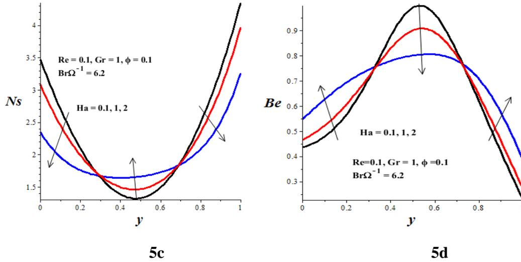
**Figure 5:** Effect of Hartmann number on a) velocity, b) temperature c) entropy generation rate, d) Bejan number
