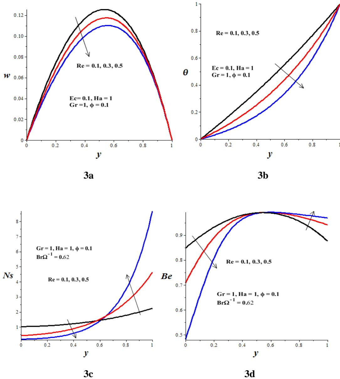
**Figure 3:** Effect of suction/injection Reynolds number on a) velocity, b) temperature c) entropy generation rate, d) Bejan number
