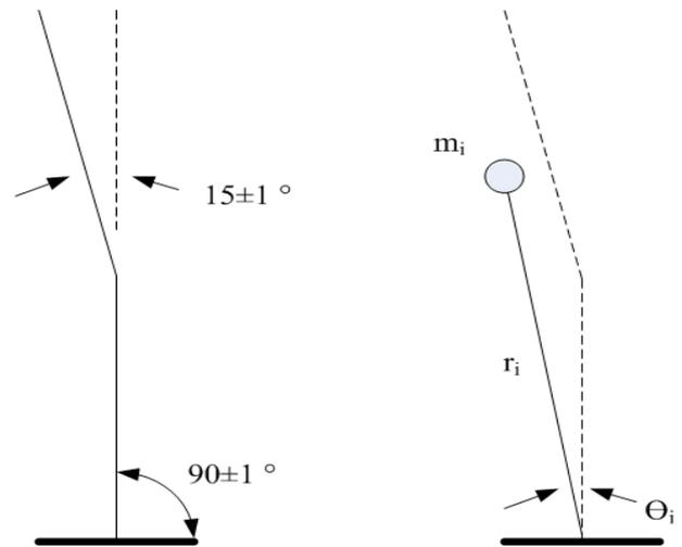
Figure 7. Schematic of mass representing each fan blade
