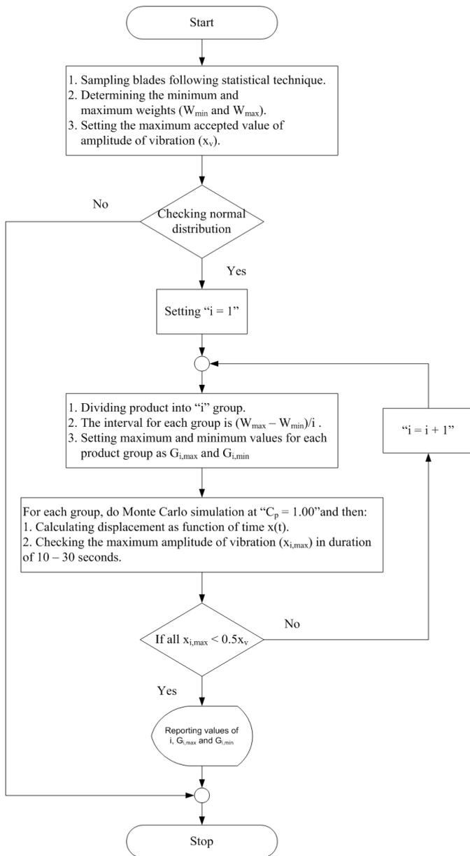
**Figure 8.** Flow chart of new procedure for reducing the effect of variation in position and dimension of fan blade in rice harvester and combine harvester
