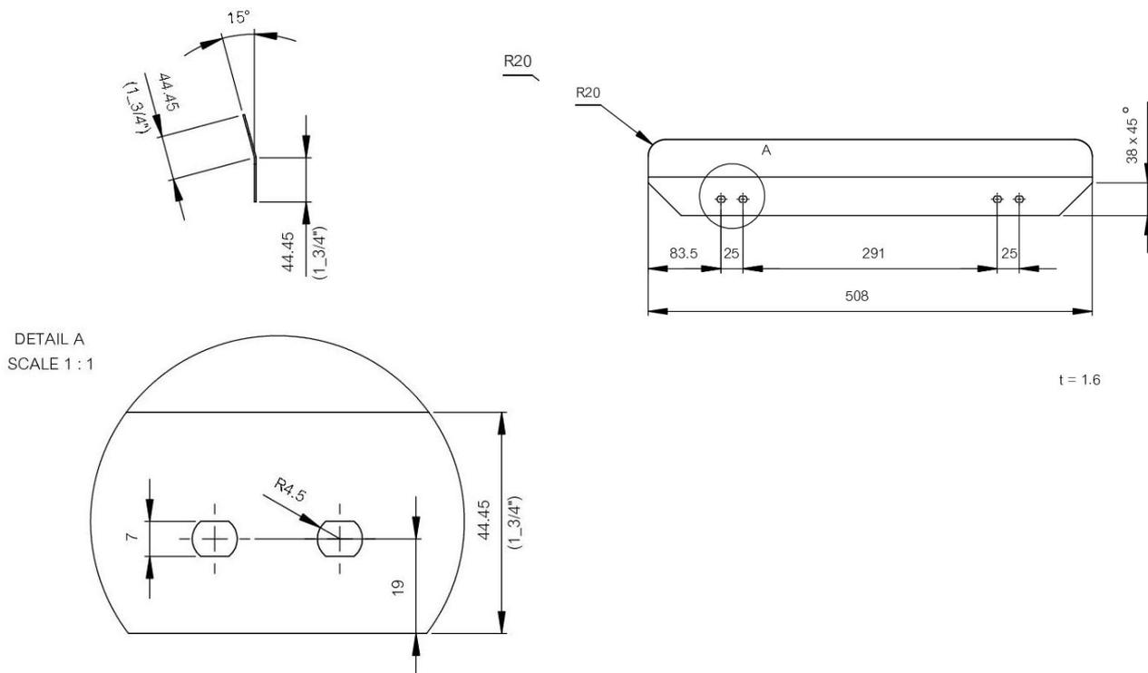
**Figure 4.** Drawing of each fan blade
