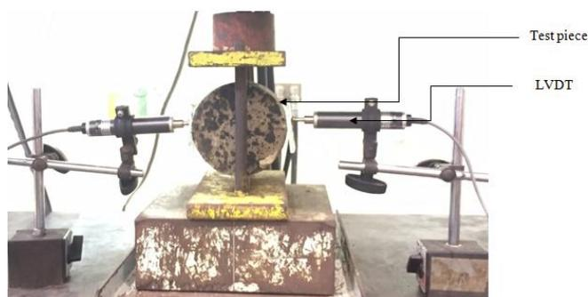
**Figure 4.** Indirect tensile strength equipment
