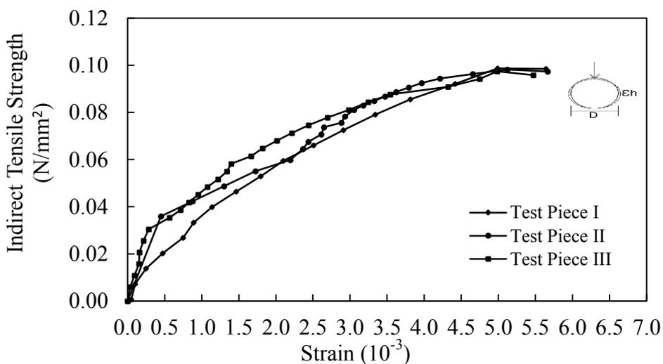
**Figure 10.** Indirect tensile strength-strain of asphalt emulsion mixture with 5% BGA
