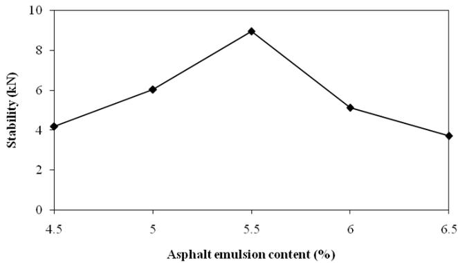
**Figure 5.** Relationship between asphalt emulsion content with stability
