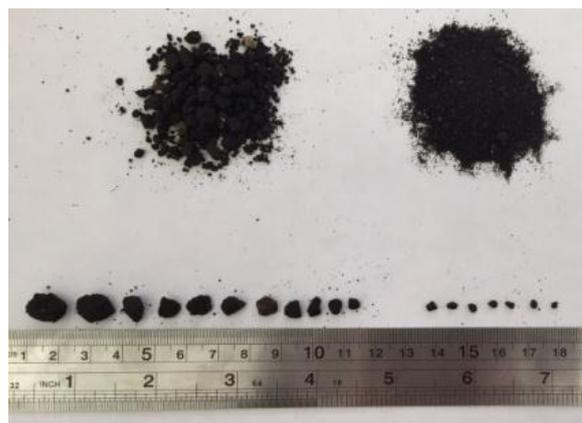
**Figure 1.** Buton Granular Asphalt BGA (dimension in mm)
