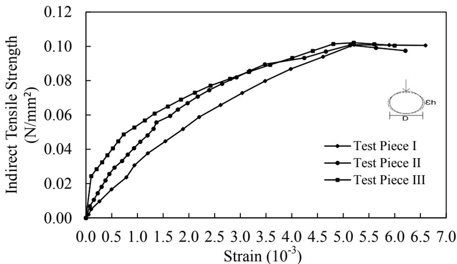
**Figure 11.** Indirect tensile strength-strain of asphalt emulsion mixture with 7.5% BGA
