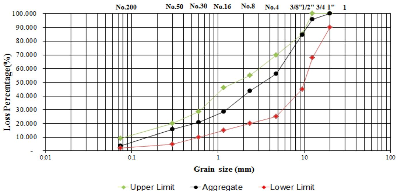
**Figure 2.** Combined aggregates gradation
