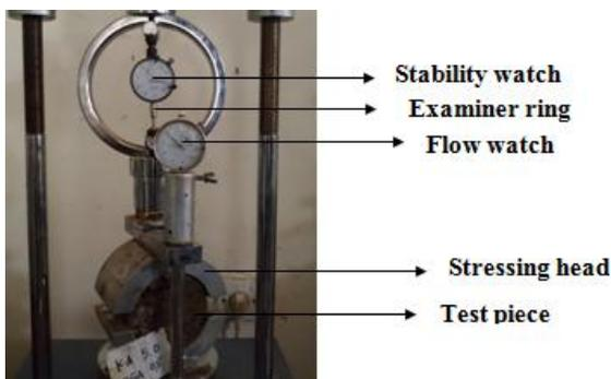
**Figure 3.** Marshall stability test equipment
