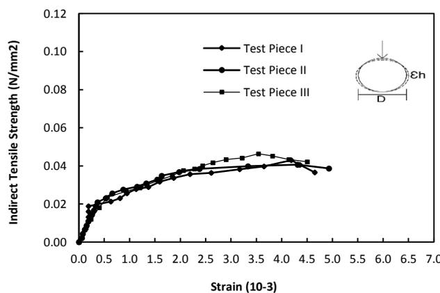
**Figure 8.** Indirect tensile strength-strain of asphalt emulsion mixture without BGA
