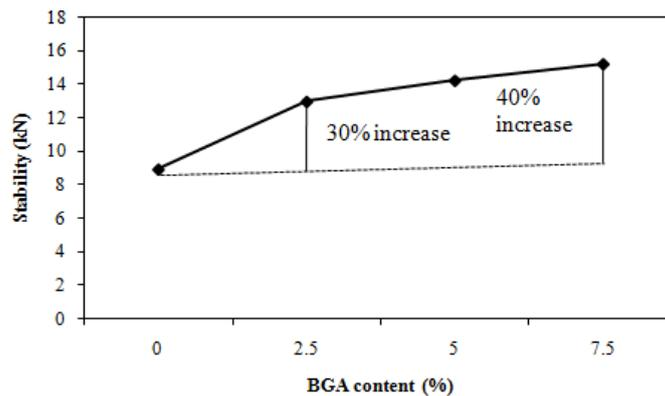
**Figure 6.** Relationship of BGA content with stability
