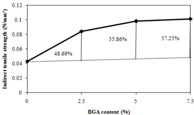
**Figure 7.** Relationship between BGA with IDT strength
