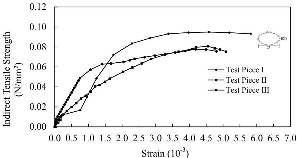
**Figure 9.** Indirect tensile strength-strain of asphalt emulsion mixture with 2,5% BGA
