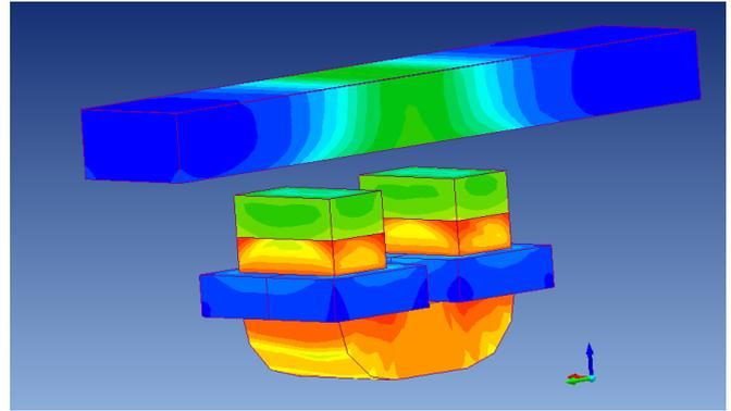
**Figure 3.** 3-D model of electromagnetic suspension
