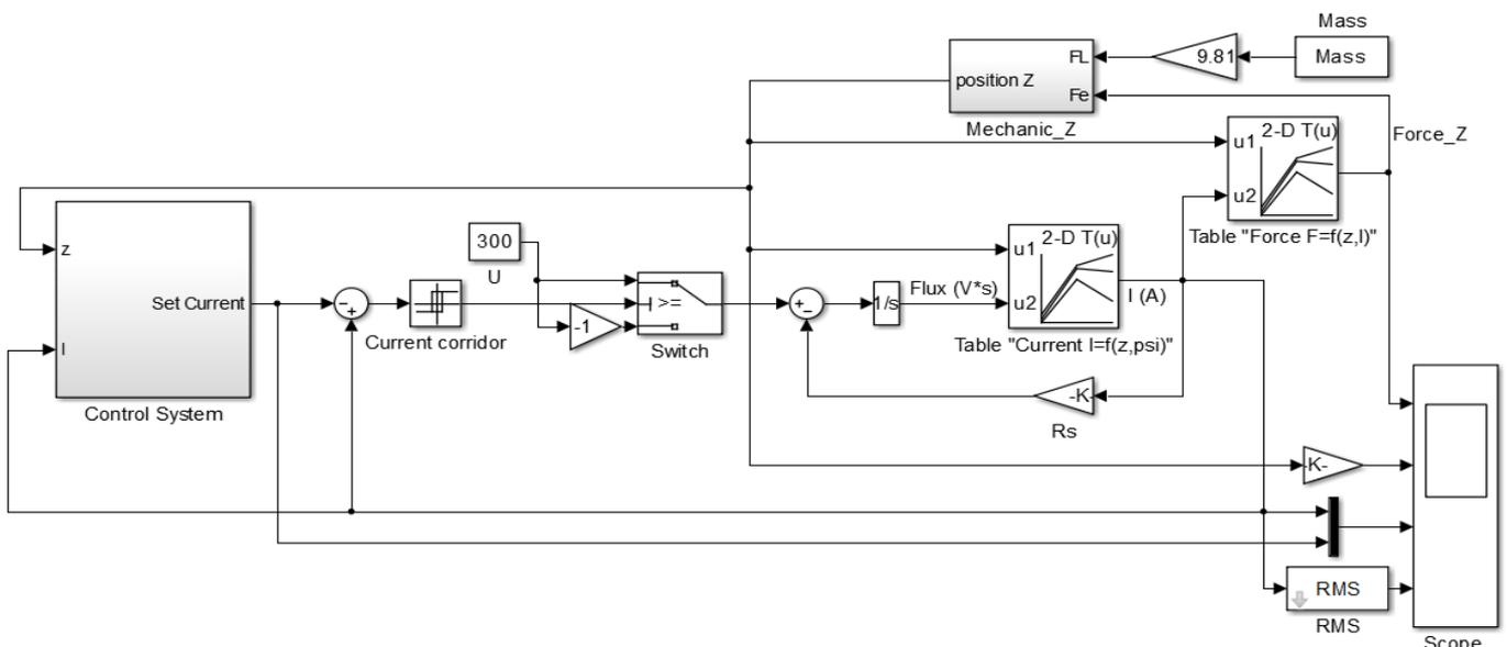
**Figure 7.** The computer model of the electromagnetic module
