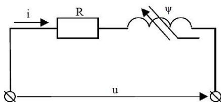
**Figure 6.** Substitution scheme of electromagnetic suspension
