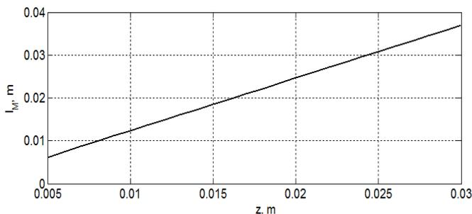
**Figure 2.** The dependency of the permanent magnet thickness on the operating gap nominal value
