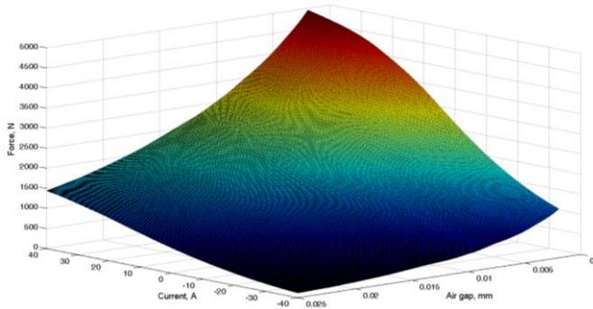
**Figure 5.** The dependency of the lifting force on the current flowing in the electromagnet and air gap coils
