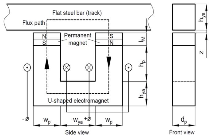
$w_p$ ,  $h_p$ ,  $d_p$  – width, height and thickness of the electromagnet pole;  $w_{ya}$ ,  $h_{ya}$  – width and height of the electromagnet core;  $h_{ys}$  – height of the flat steel bar (track);  $l_M$  – permanent magnet thickness;  $z$  – air gap.
