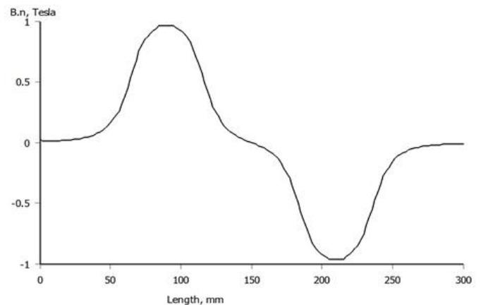
**Figure 4.** The distribution of magnetic flux density above electromagnetic suspension poles
