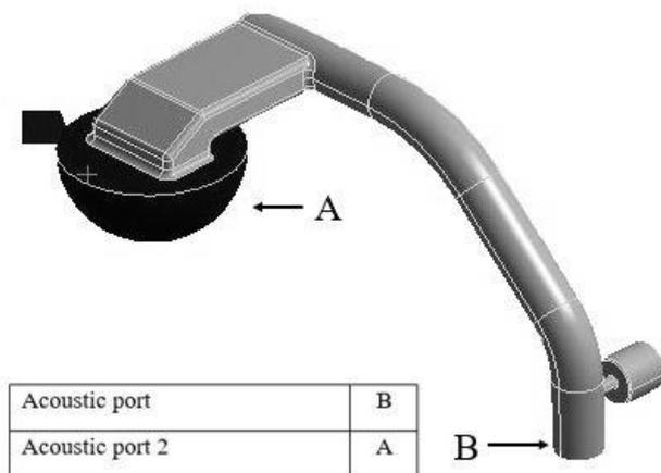
**Figure 4:** Position for boundary condition of analysis model
