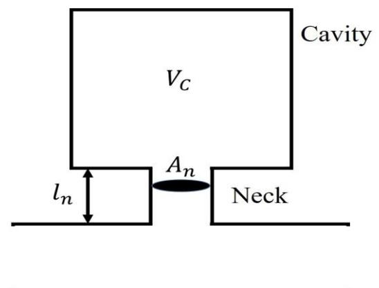
Figure 1: Schematic of a typical Helmholtz resonator
