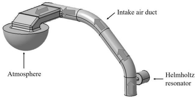
**Figure 3:** Intake system model with resonator
