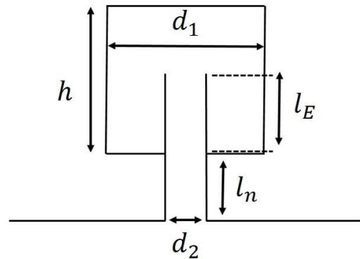
Figure 2: Schematic of a Helmholtz resonator
