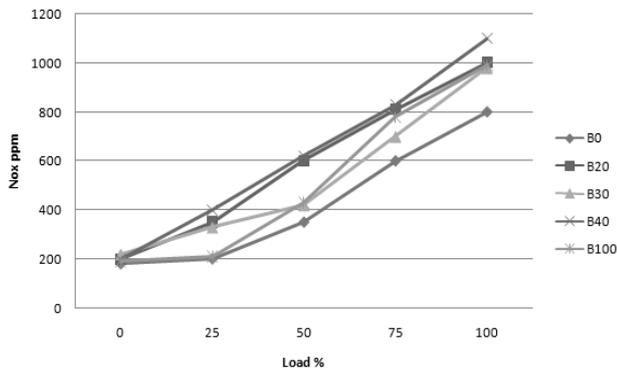
**Figure 4:** NO<sub>x</sub> emissions with varying loads of different blends.[16]
