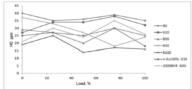
**Figure 2:** HC emissions with varying loads of different blends[8].
