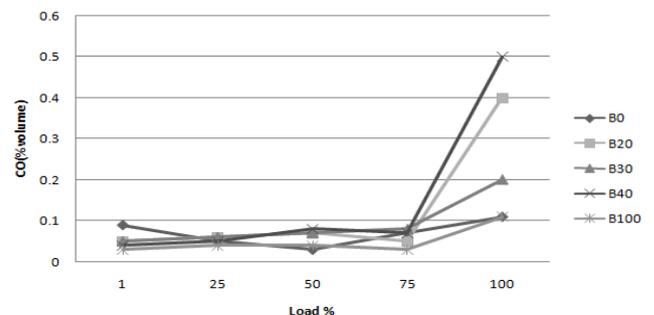
**Figure 3:** CO emissions with varying loads of different blends.[8]
