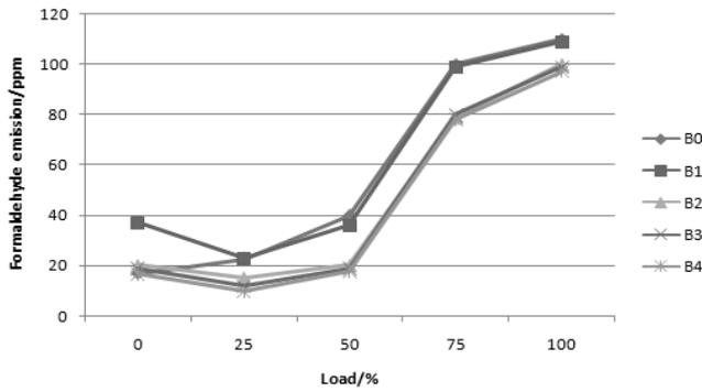
**Figure 6:** Effect of biodiesel and engine load on formaldehyde emission.[4]
