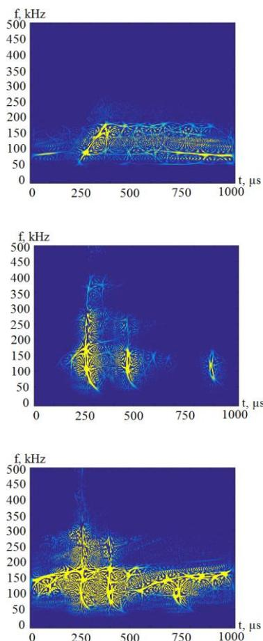
**Figure 4.** Examples of acoustic signals caused by the destruction of material in frequency domain.
