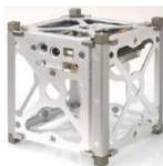
**Figure 1:** CubeSat Structure.
