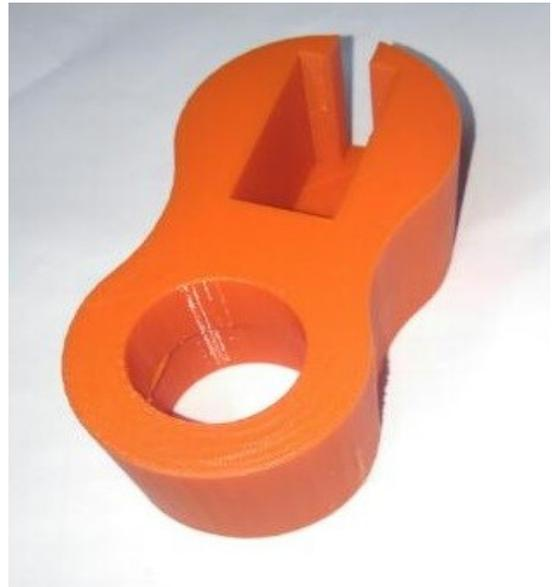
**Figure 4:** A 3D printed leg for the proposed robot. The upper rectangular slot is for fitting a servo motor while the lower circular slot is for fitting D.C. motor
