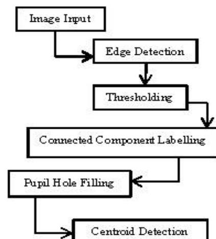
Figure 1: System for Noise Removal and Feature Extraction
