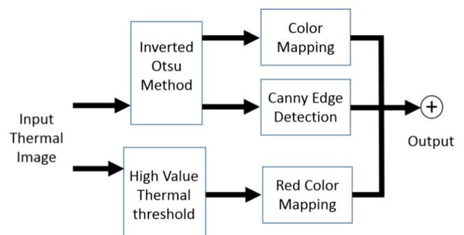
Figure 1: Algorithm of Enhanced-Color Mapping Algorithm
