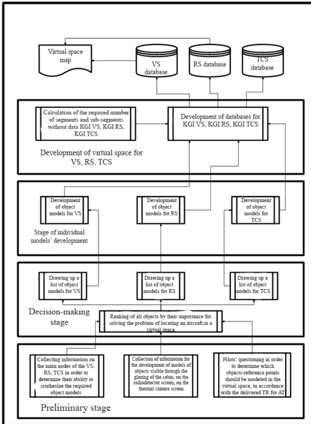
**Figure 4:** Stages of information preparation for a visual simulator, radiodetector simulator, thermal camera simulator.
