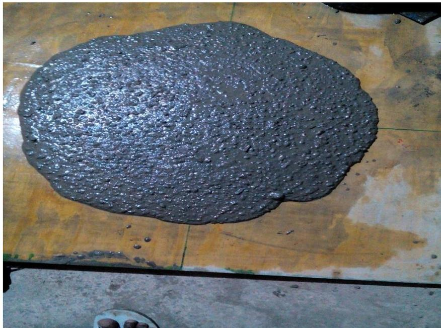
Figure 1: Slump flow test
