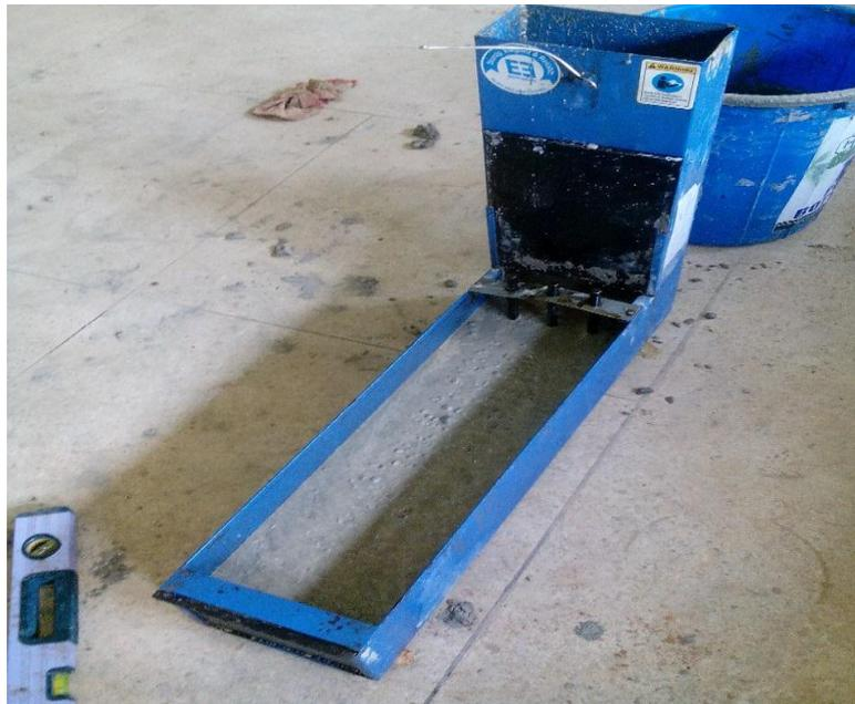
**Figure 6:** L-box test
