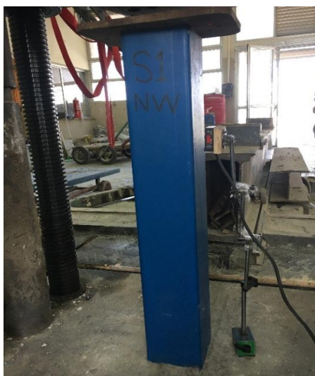
Figure 3: Column specimen test setup
