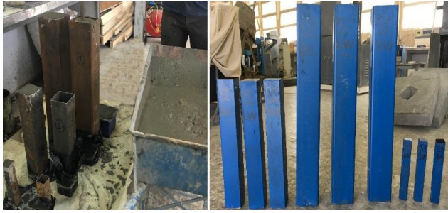
Figure 2: Casting of concrete and preparing for column specimens
