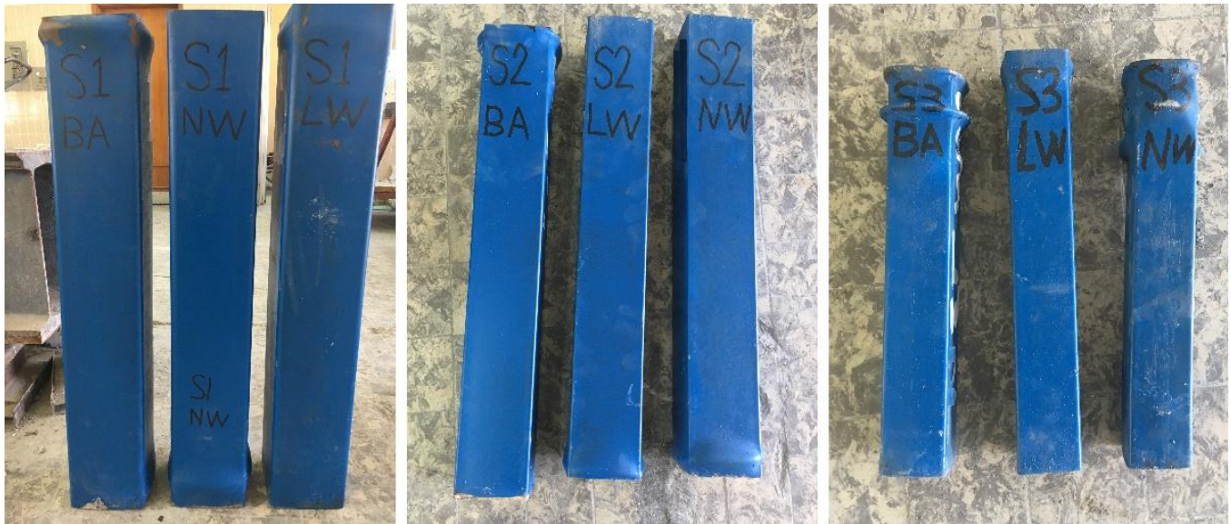
Figure 4: Modes of failure for tested column specimens
