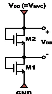
Figure 4: Conventional body bias generation with diode-connected MOSFET voltage divider.
