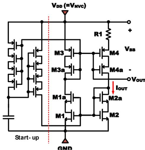
Figure 5: Proposed body bias generation with beta-multiplier reference circuit.
