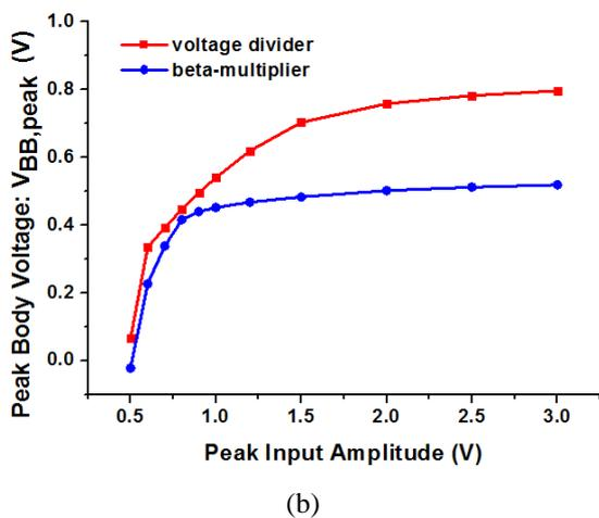
**Figure 8:** (a) Average body voltage, (b) Peak body voltage versus input voltage.
