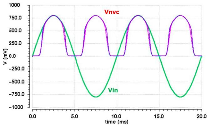
**Figure 10:** NVC output waveforms with a sinusoidal 0.8 V input at 100 Hz and loaded with a 100 kΩ resistor.
