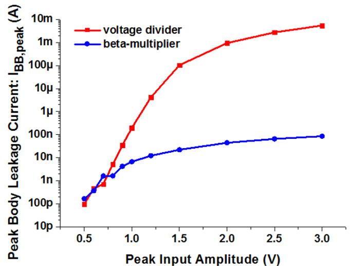
**Figure 9:** (a) Average body leakage current, (b) Peak body leakage current versus input voltage.
