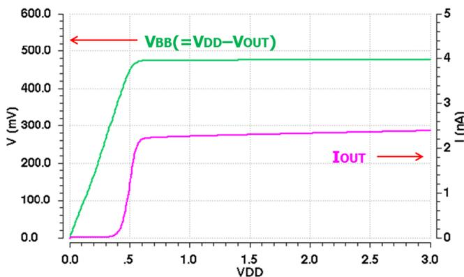
Figure 6: Supply voltage dependence of the output voltage and current.
