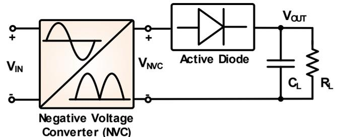
Figure 1: Block diagram of two-stage FWR.
