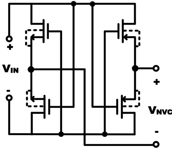
Figure 2: Schematic of basic negative voltage converter.
