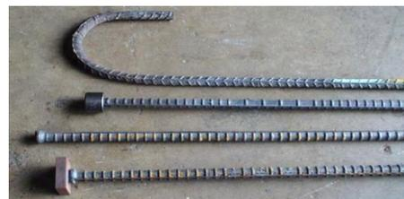
**Figure 3:** Different headed bars and hooks bars
