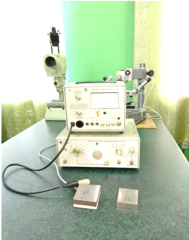
Figure 1: Pilot plant for measuring contact-potential difference, V_c
