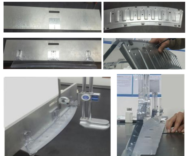
Figure 3: Combination and measurement of OLED TV stand neck and jig
