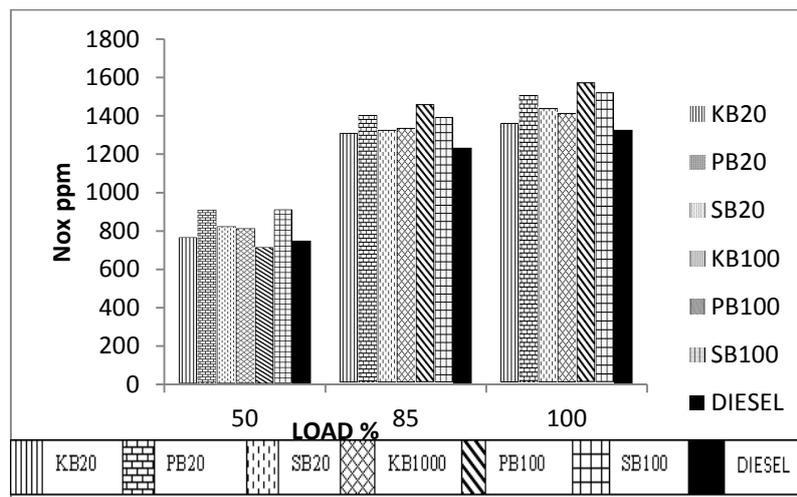
Figure 6. NOx Emissions vs. load for different blends
