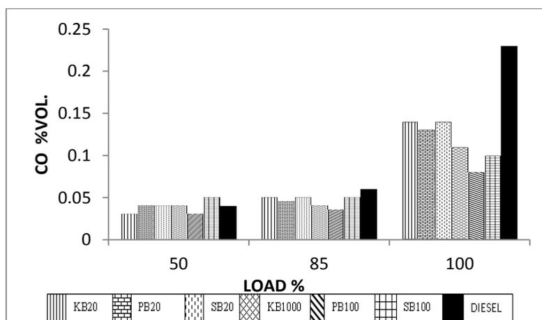
Figure 4 carbon monoxide emissions vs. load for different blends
