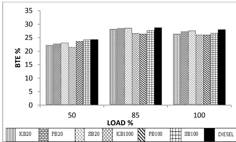
Figure 2 BTE vs. Load for various biodiesel blends.
