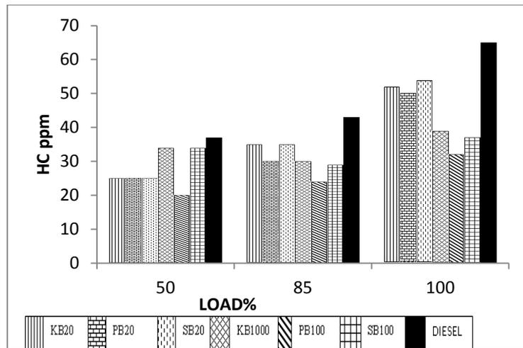
Figure 5 Unburnt hydrocarbon emissions vs. load for different blends
