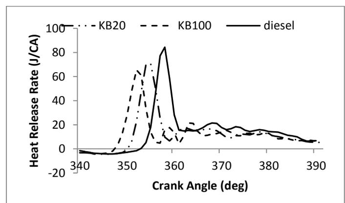
**Figure 9.** Variation of heat release rate with crank angle at 85% load for KB blends
