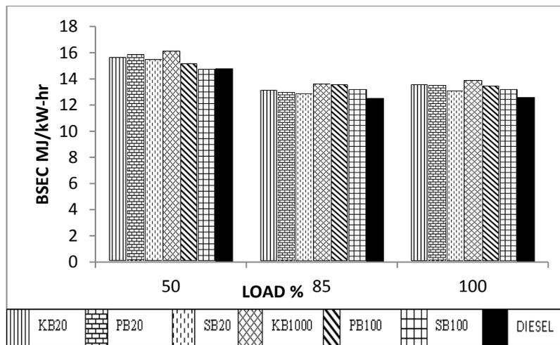
Figure 3 BSEC vs Load for various biodiesel blends.
