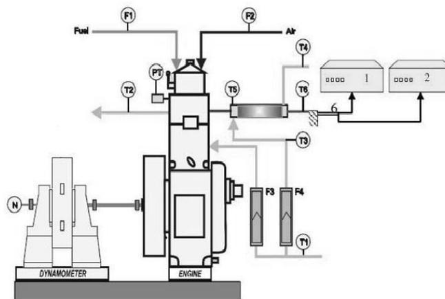
**Figure 1.** Schematic diagram of experimental set up of engine test rig
