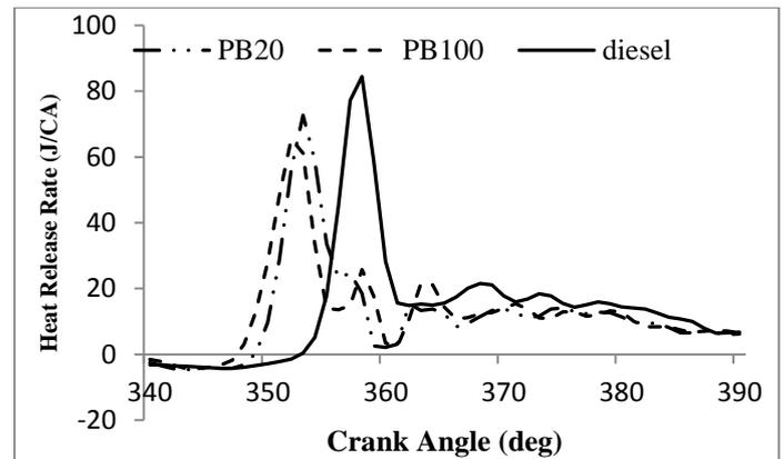
**Figure 8.** Variation of heat release rate with crank angle at 85% load for PB blends
