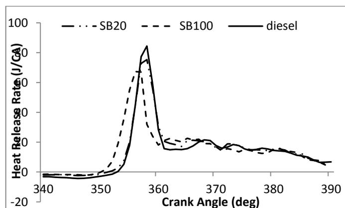
**Figure 7.** Variation of heat release rate with crank angle at 85% load for SB blends
