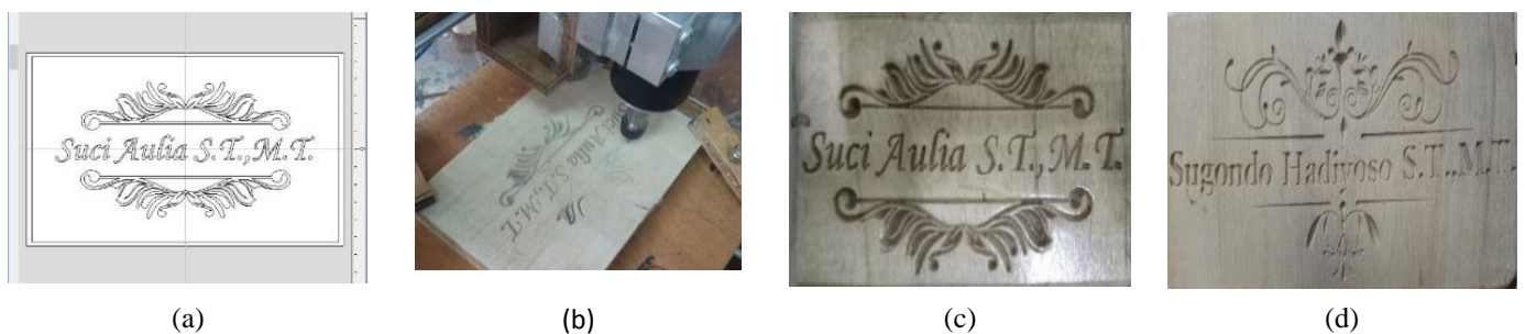
(a) (b) (c) (d) Figure 6: (a)Image design. (b)Engraving process. (c)Engraving result. (d)Engraving result.
