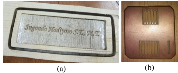
Figure 7. (a) Marking result on wood board. (b) Marking result on PCB.
