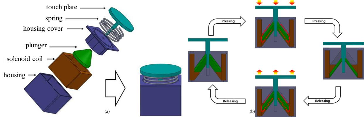
**Figure 4:** Schematic illustration of the stiffness tuning part and its operating principle.
