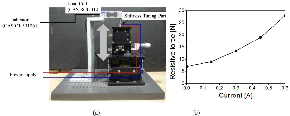
**Figure 6:** Experimental setup to measure the generated force of the developed stiffness tuning module and its result.
