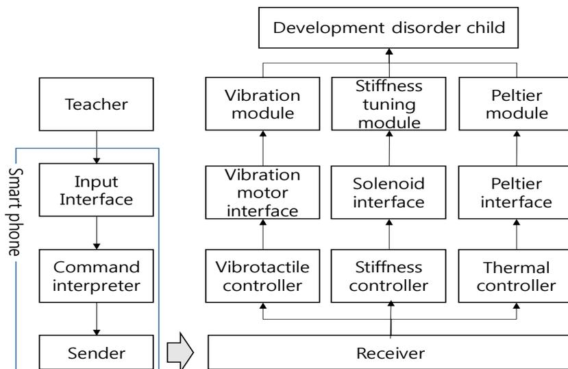
**Figure 3:** Signal flow of the proposed system
