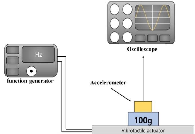
**Figure 5:** Experimental setup to measure vibrational force of the vibration module
