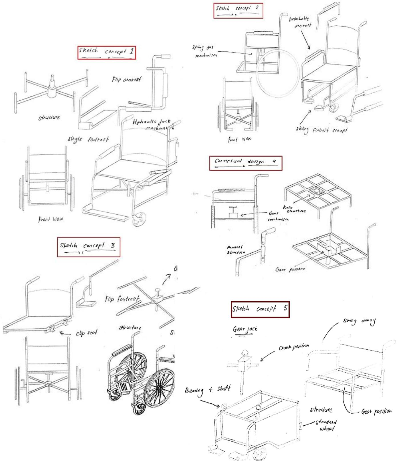
Figure 2: Design concept of manual wheelchair
