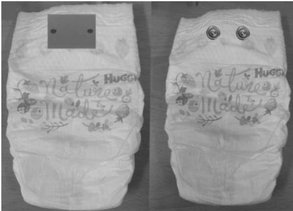
**Figure 8.** Wet detector fixed with diaper using pressing studs
