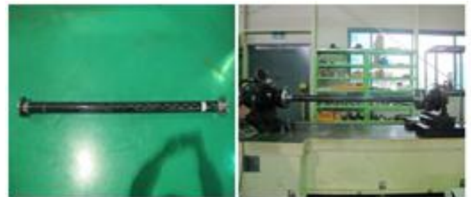
Figure 9: Torsional strength testing device
