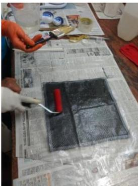
Figure 1: Hand lay-up process
