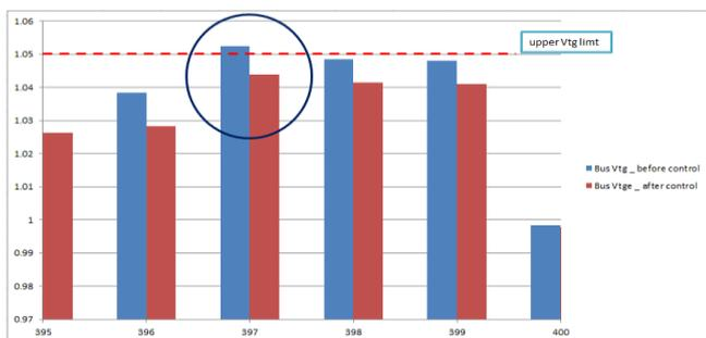
**Figure 5:** Voltage profiles before and after voltage control
