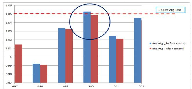
**Figure 6:** Voltage profiles before and after voltage control
