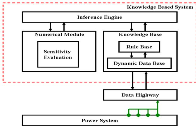
Figure 1: Structure of intelligent voltage control system
