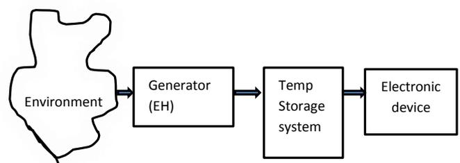
**Figure 1:** Energy harvesting as alternative for micro powering
