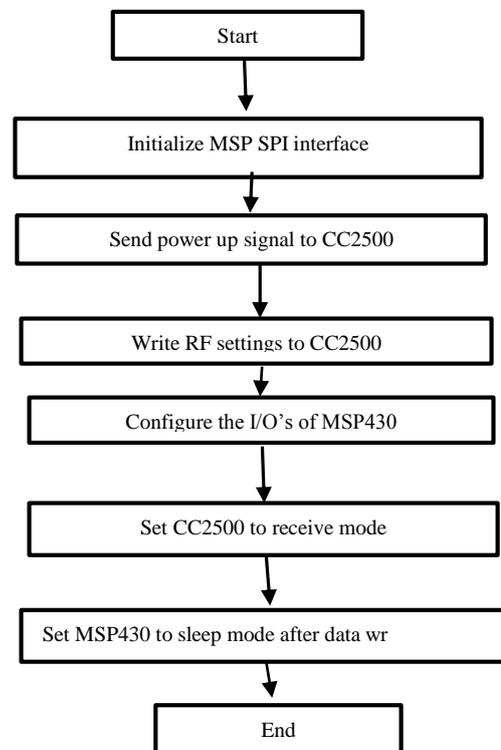
Figure 8: flow chart for interfacing CC2500 with MSP430.
