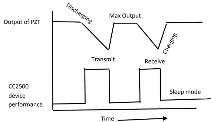
**Figure 9:** Output Vs Device performance
