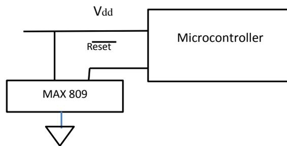
**Figure 10:** A three terminal supervisory IC with voltage monitoring
