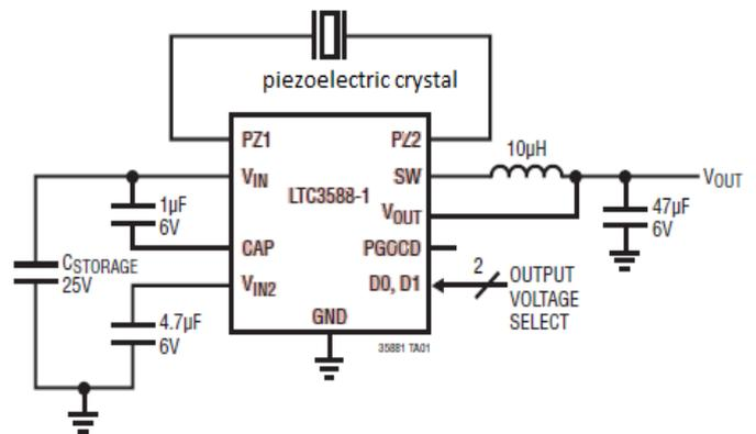
Figure 4: Technique for harvesting energy
