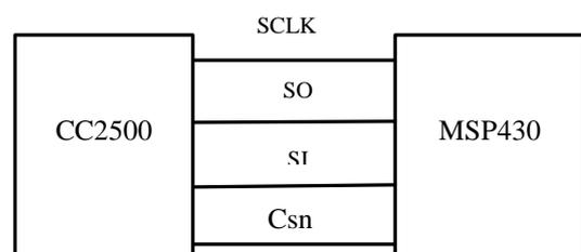
**Figure 6:** Interfacing of CC2500 with microcontroller MSP430
