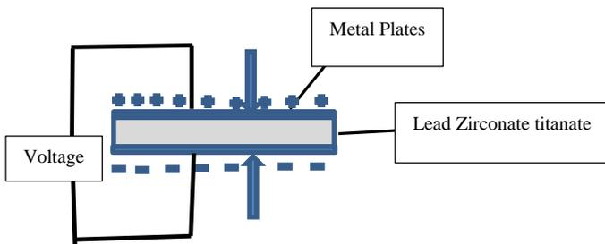
Figure 3: Compressing produces energy
