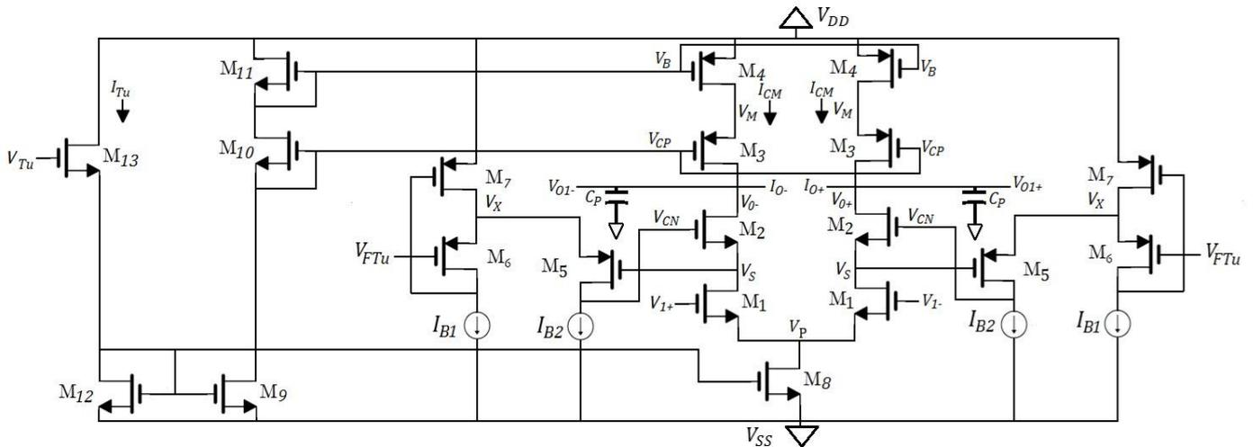
**Figure 6: Proposed Transconductor**
