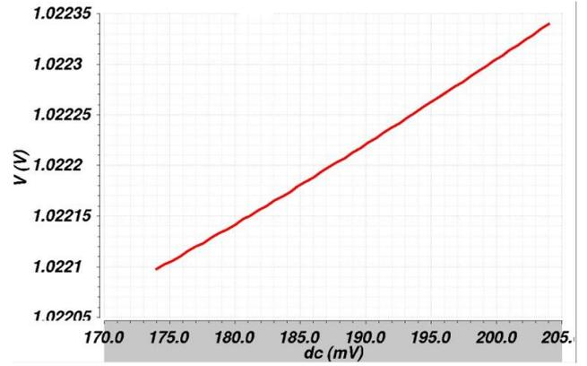
Figure 11: Output Gain vs Fine Tuning (VFTu) Voltage
