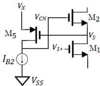
Figure 3: Gate driven gain boosting circuit
