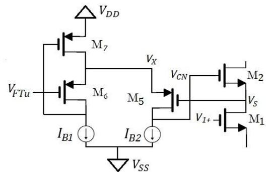
Figure 4: LFA amplifier
