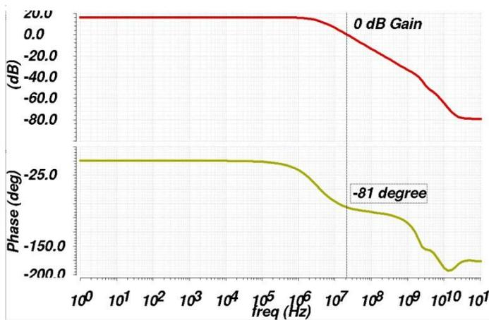
Figure 9: Gain and Phase curve
