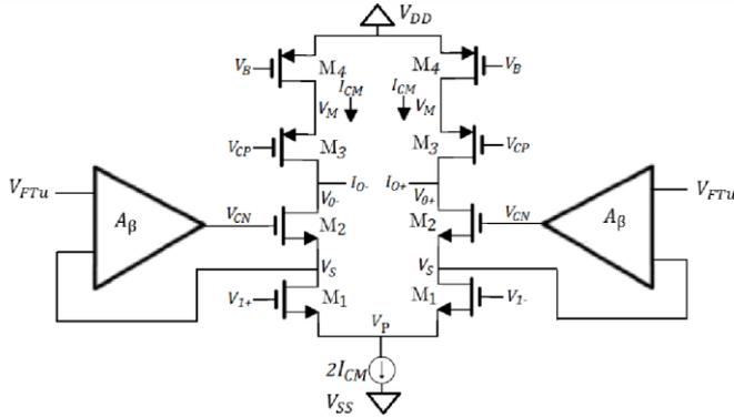
**Figure 1:** Operational Transconductance Amplifier (OTA)
