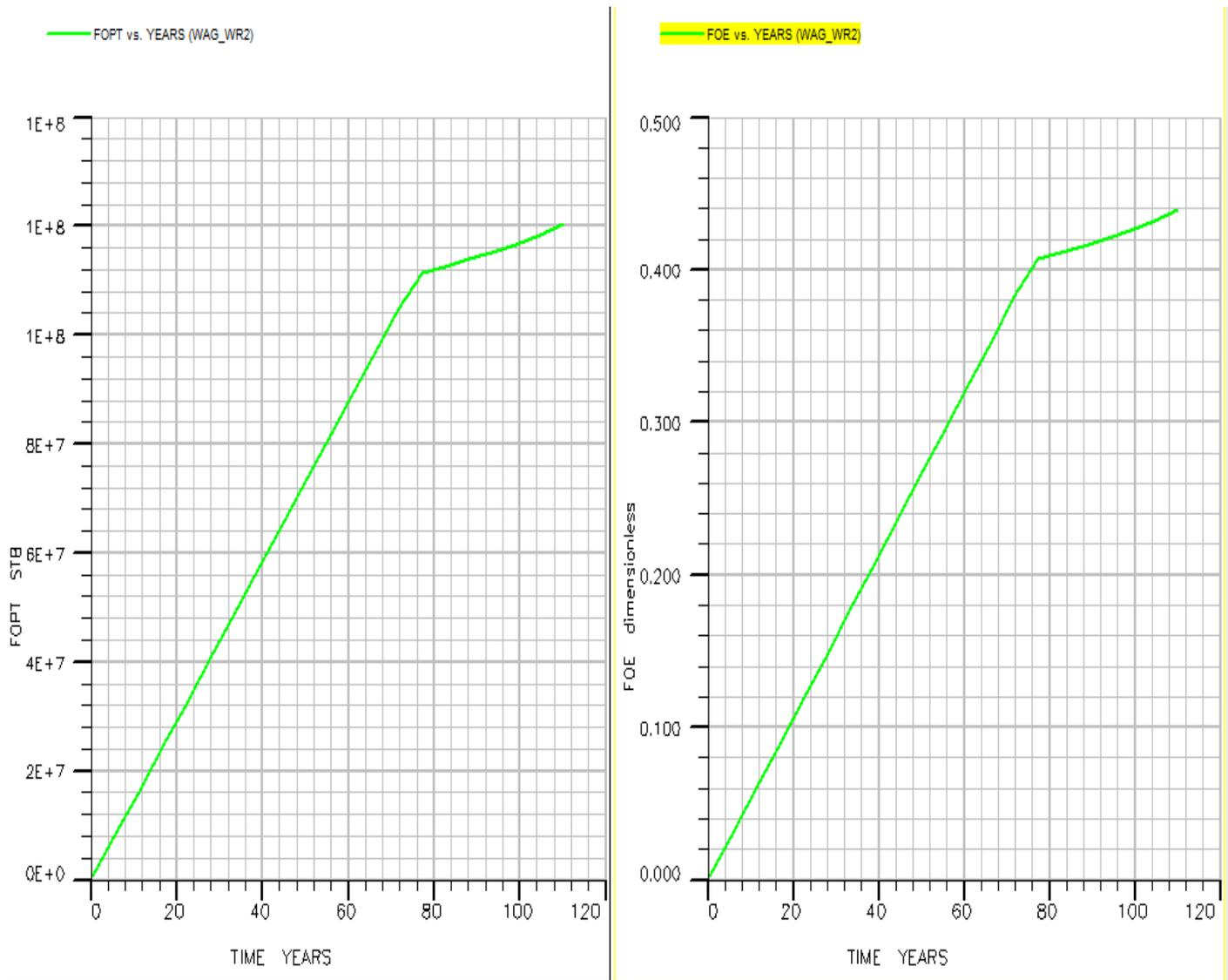
Figure 7: Plots FOPT, FOE VS time using MWAG (2:1)
