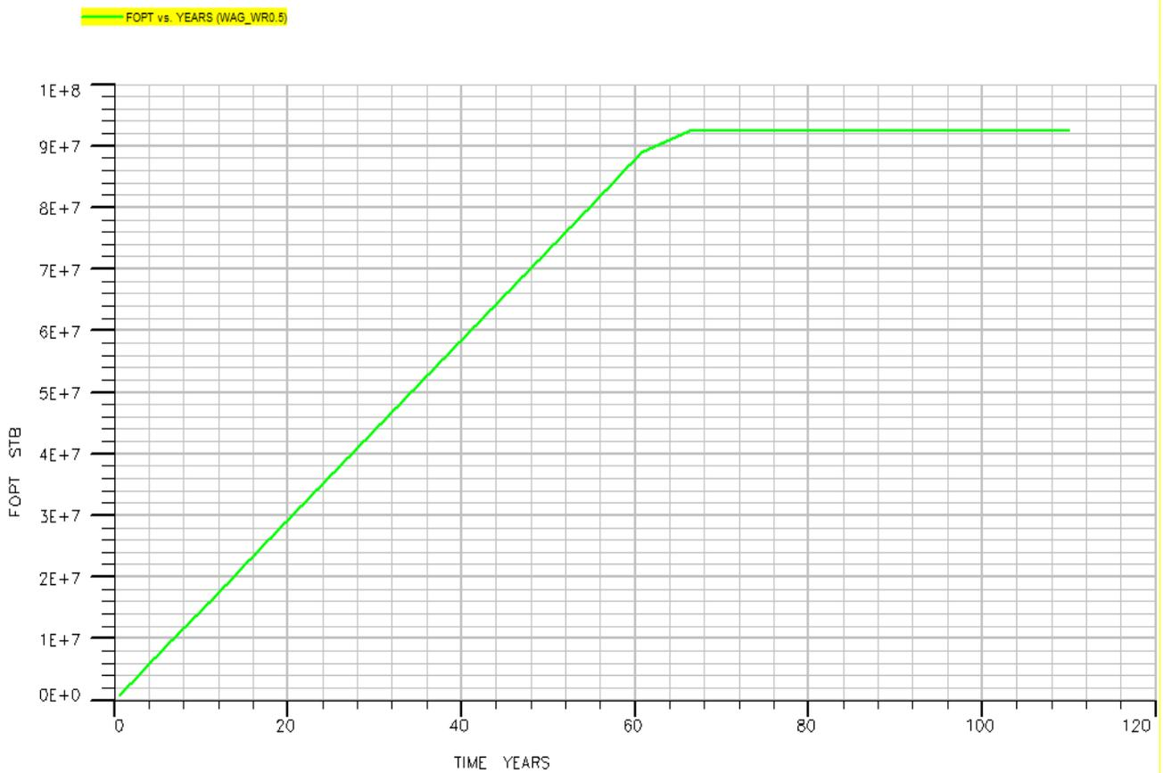
**Figure 10:** Showing FOPT VS time using MWAG (1:2)
