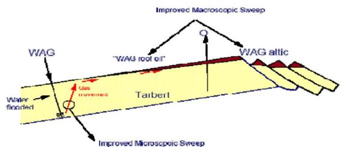
**Figure 1:** WAG process (accessibility of WAG to difficult to reach oil) (Esmail, 2005).
