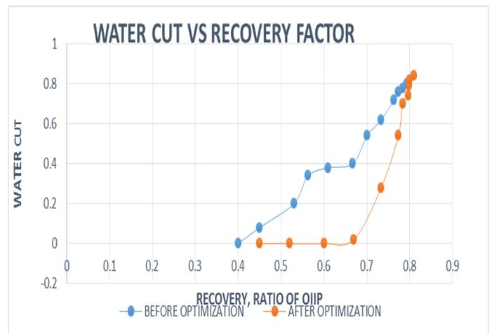
**Figure 16:** Plots showing WATER CUT VS RECOVERY FACTOR before and after optimization
