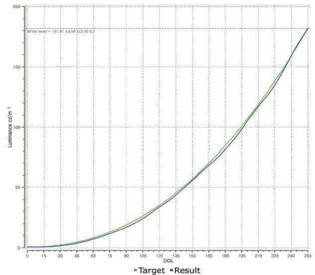
Figure 4. A gamma curve by the proposed calibration algorithm
