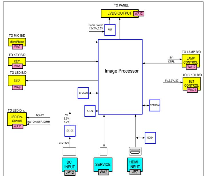
Figure 2. A block diagram of the proposed SIPCB architecture
