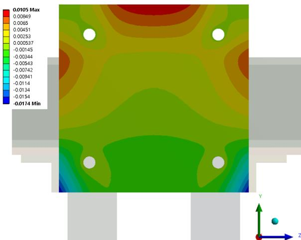
Figure 8: X-deformation ( $U_x$ ) distribution
