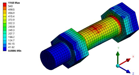
**Figure 11:** Von Mises stress distribution of the lower bolt
