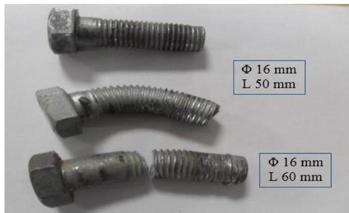
**Figure 5:** The fastening bolts broken by the accident
