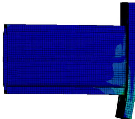
**Figure 12:** The deformed connecting end of the boom head shown in FEA
