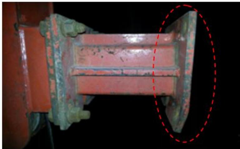
**Figure 4:** The deformed connecting end of the boom head
