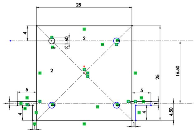
Figure 9: The end plate of the bucket-type work platform
