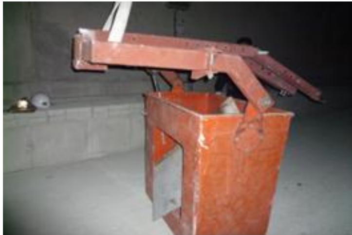
**Figure 3:** The bucket-type work platform fell down
