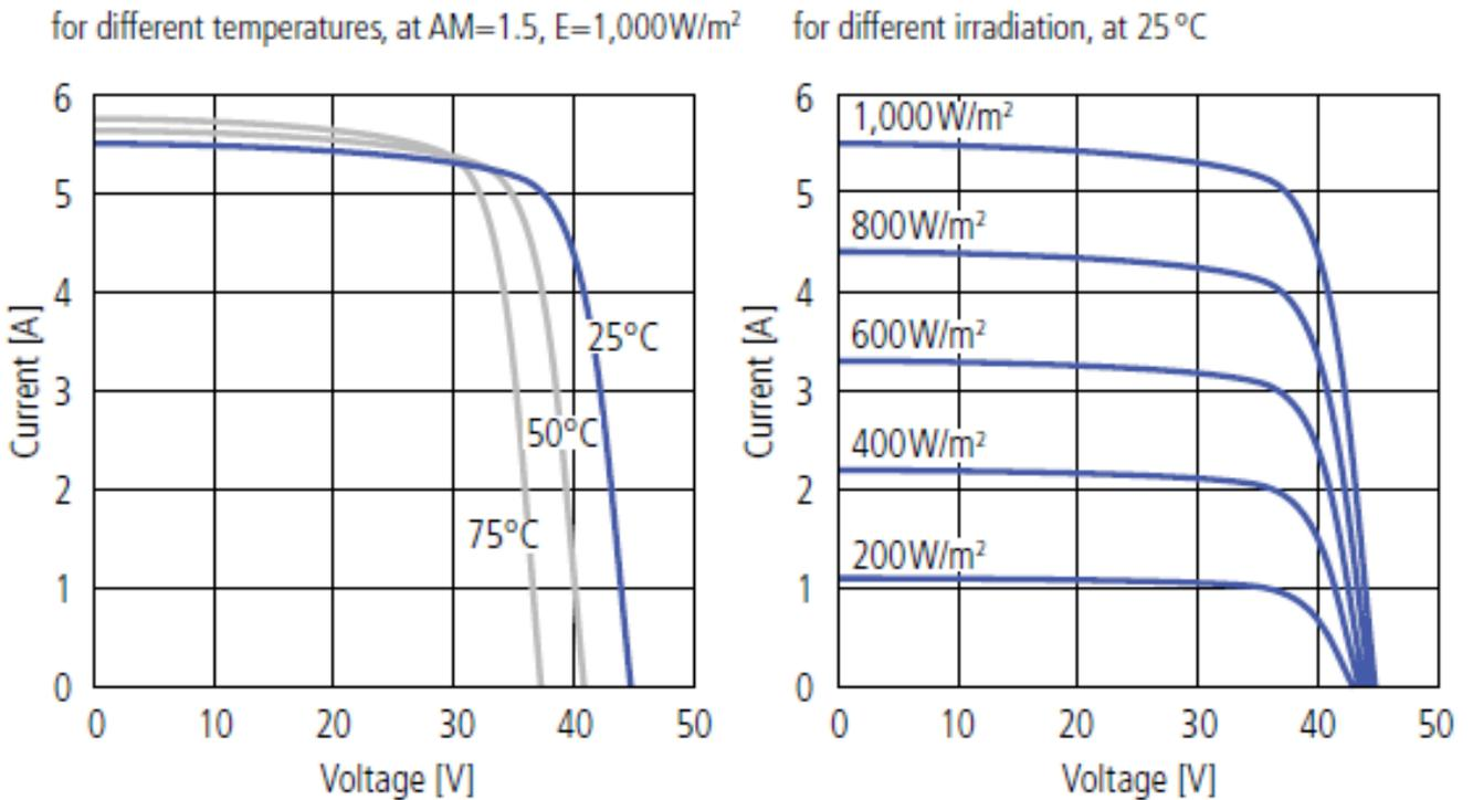
**Figure 10:** I-V curve of the PV module for different irradiation levels and different temperatures [40].
