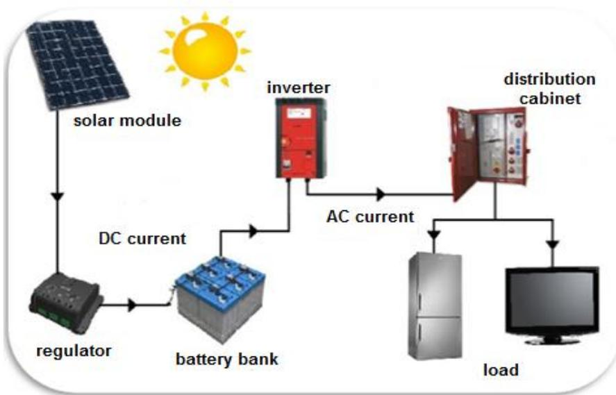
**Figure 9:** A schematic diagram of a stand-alone PV system [36].
