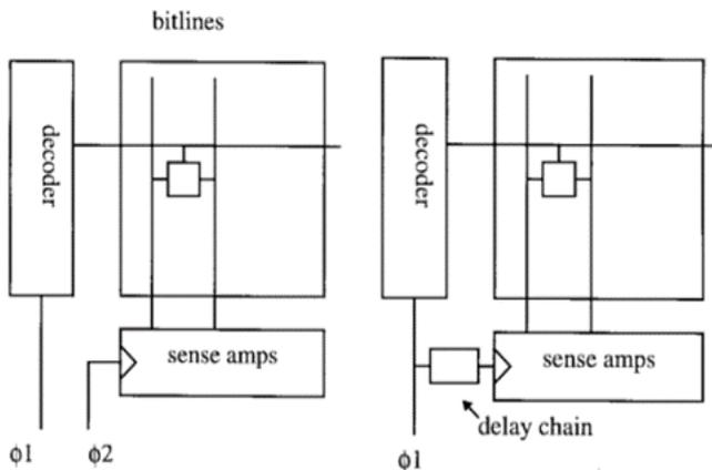
**Figure 1:** Circuit techniques for the generation of wordline and sense amplifier signal
