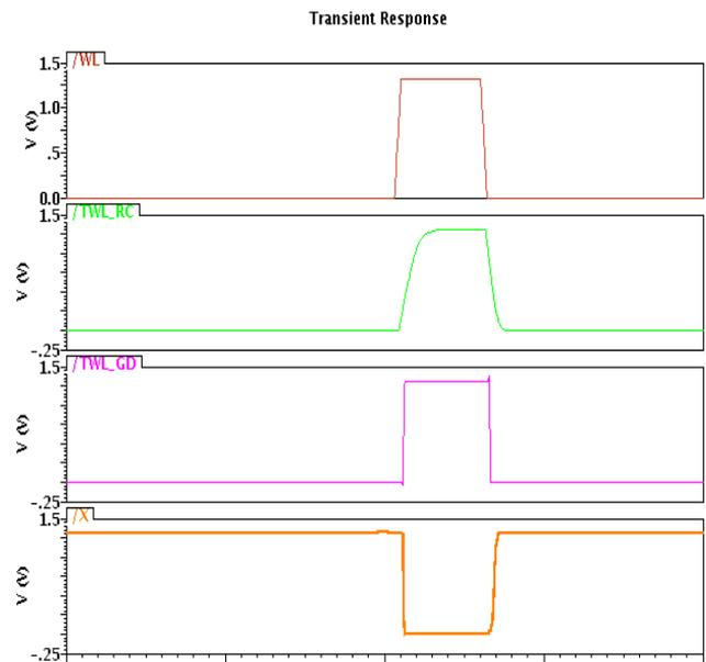
**Figure 4:** Self-time control signal (X) generation at FF/125°C/1.32V
