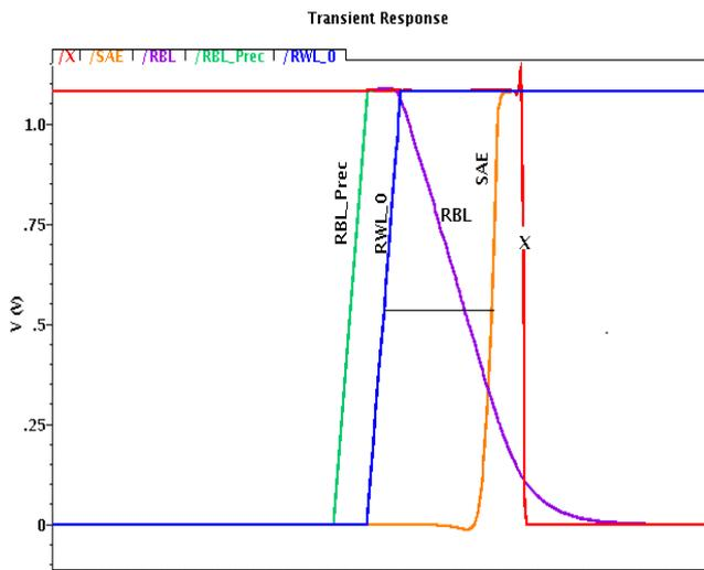
**Figure 6:** Generation of SAE signal at SS/-40°C/1.08V
