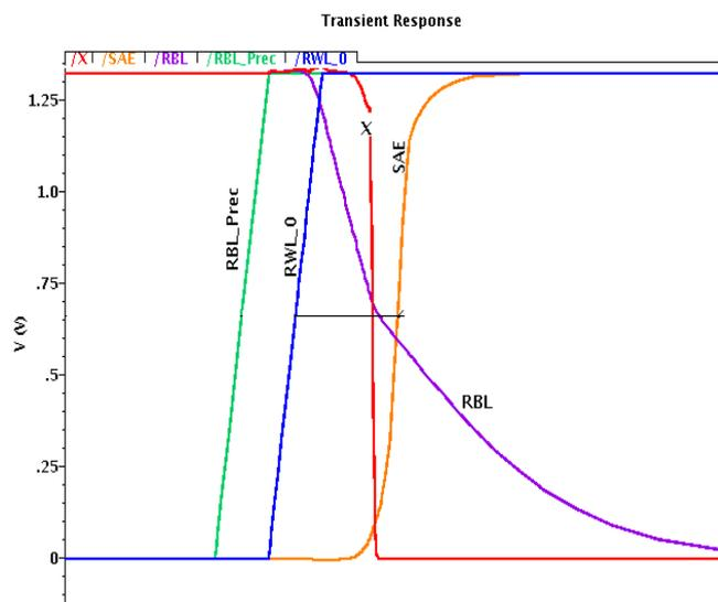
**Figure 7:** The delayed SAE signal generation at FF/125°C/1.32V
