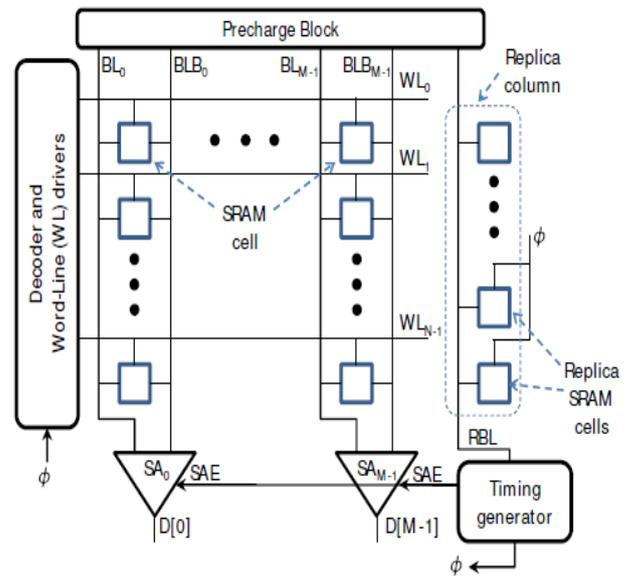
**Figure 2:** Self-time replica bit line control circuit
