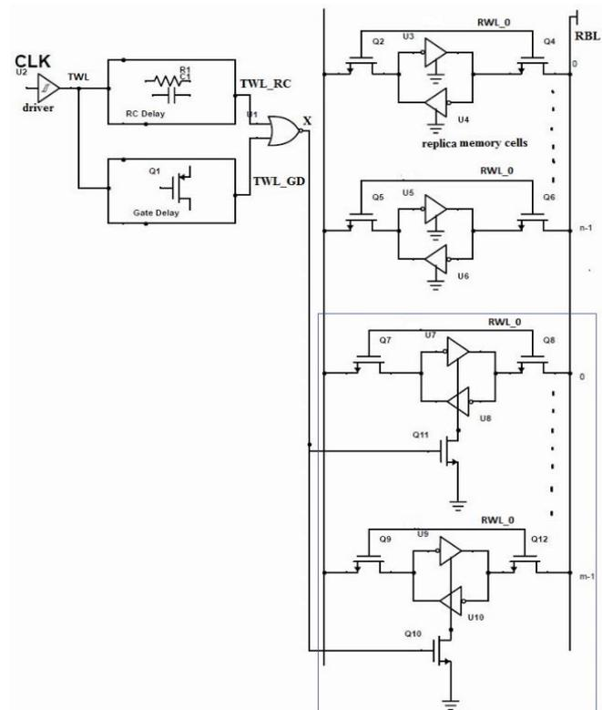
Figure 3: Proposed self-time circuit diagram
