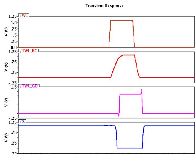
**Figure 5:** Self-time control signal (X) generation at SS/40°C/1.08V
