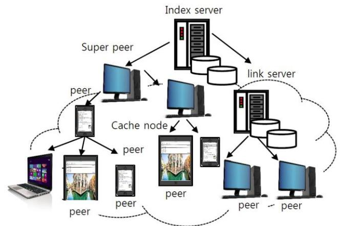
**Figure 1.** The general overview of the wire/wireless P2P systems
