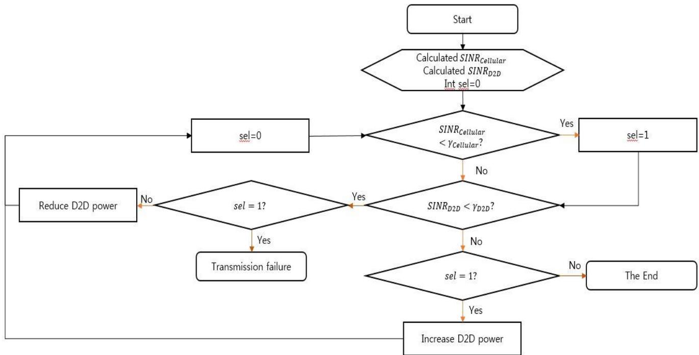
**Figure 2.** Flow chart of Power Control
