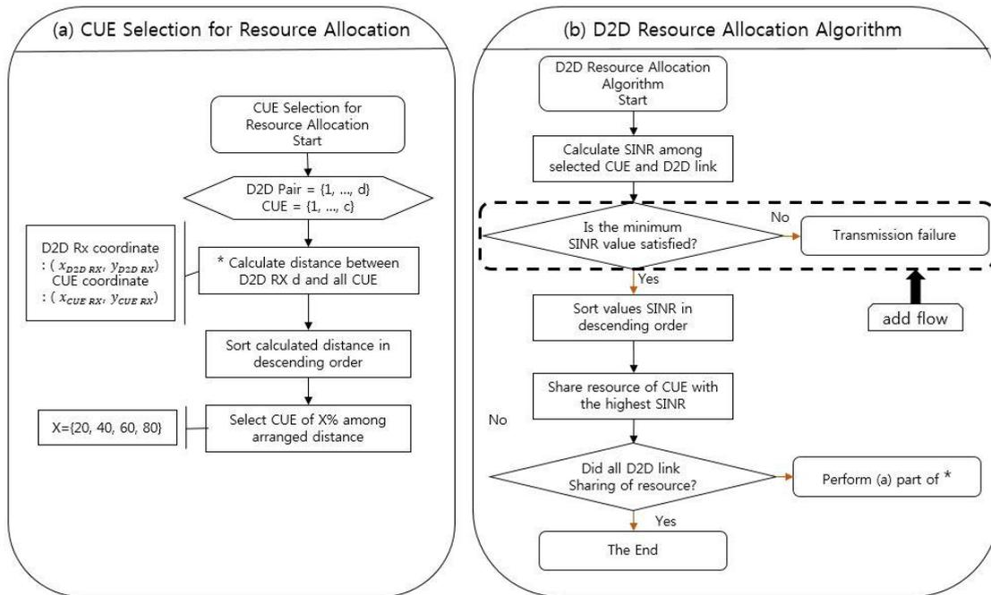
Figure 2. Flow chart of the resource allocation scheme
