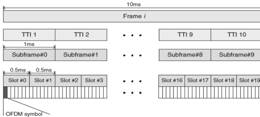
Figure. 2: Frame structure of LTE [21]
