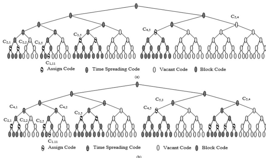
**Figure 3:** Illustration of ANC multi code assign (a)  $8R$  arrives (b)  $8R$  arrives again
