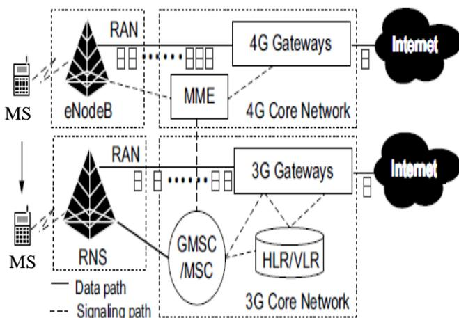
Figure. 1: Architecture of 4G-3G networks.
