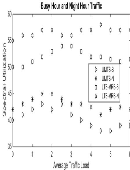
**Figure. 4:** Spectral utilization of UMTS and LTE interface in Busy and Night Hours.
