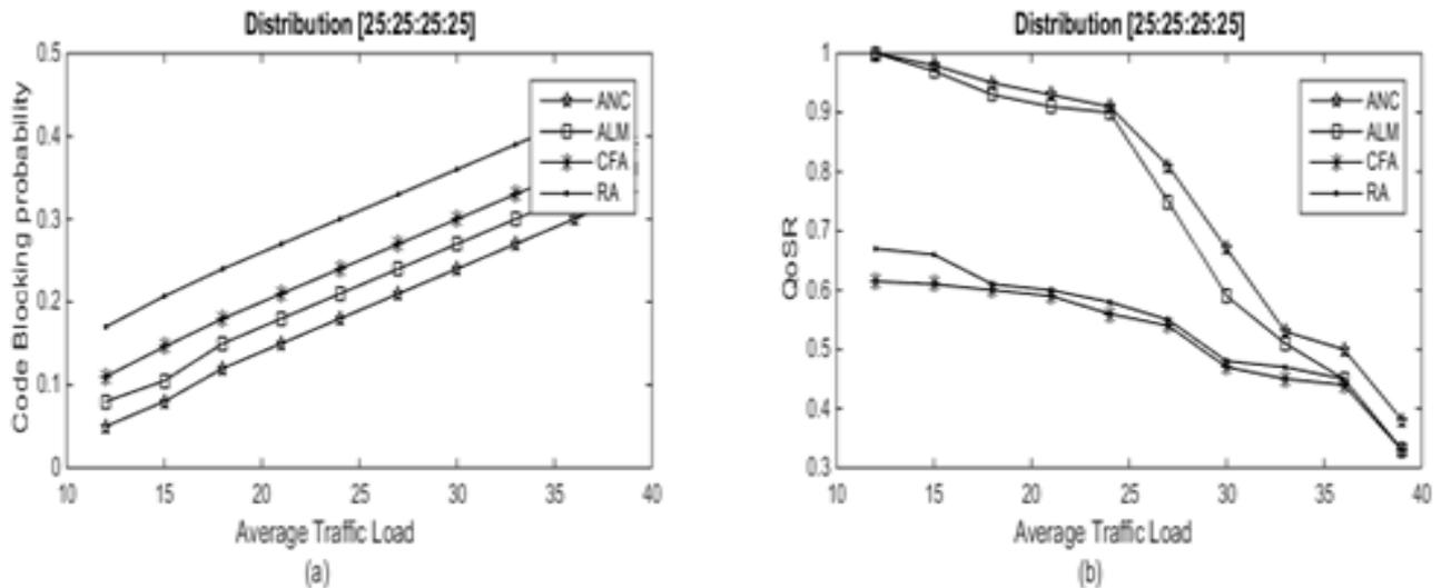
**Figure 6:** (a) Code blocking probability in presence of variable traffic load (b) QoSR in presence of variable traffic load.
