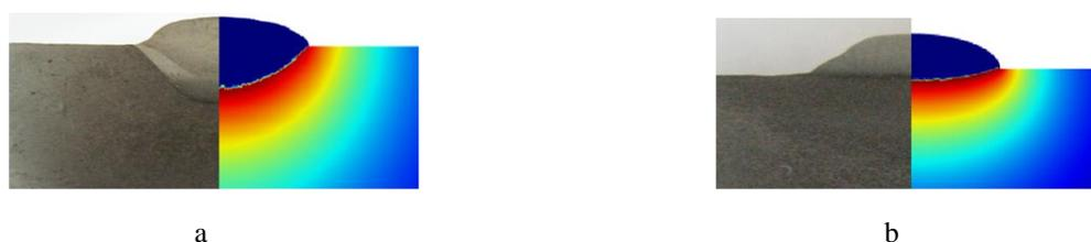
**Figure 7:** Experimental and calculated cross-sections of the weld bead in plasma surfacing at direct (a) and reverse polarity (b)
