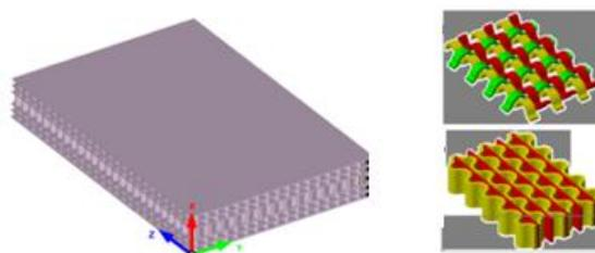
**Figure 4:** Example of FRP sandwich panels [88]
