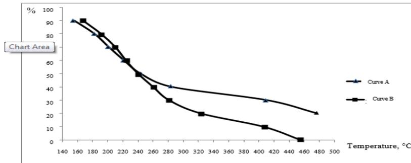
**Figure 2:** Mass-change of fuel oil sample (a) and of fuel oil sample with the addition of nickel 2-ethylhexanoate with increasing temperature.
