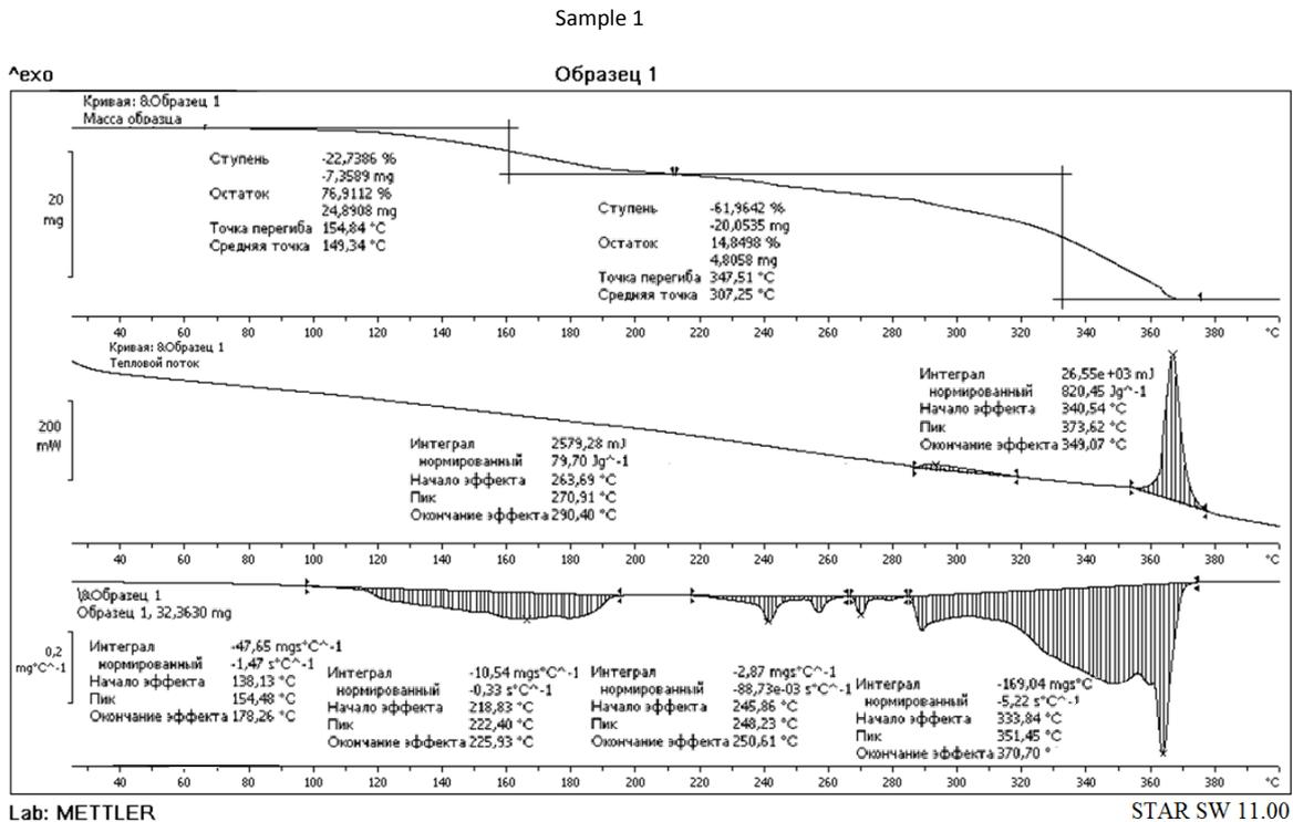
**Figure 3:** Nickel 2-ethylhexanoate sample thermogram.
