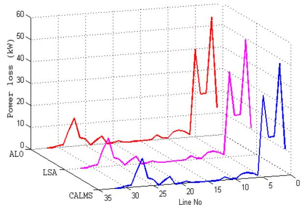
**Figure.15:** Comparison of power loss at type 3 load condition
