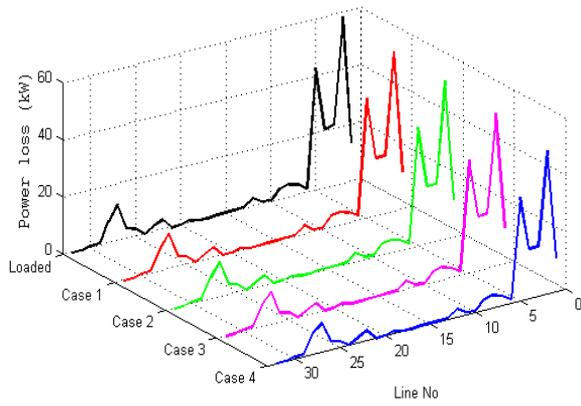
**Figure.10:** Comparison of power loss at type 1 load condition
