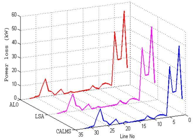
**Figure.13:** Power loss for various cases at type 1 load condition
