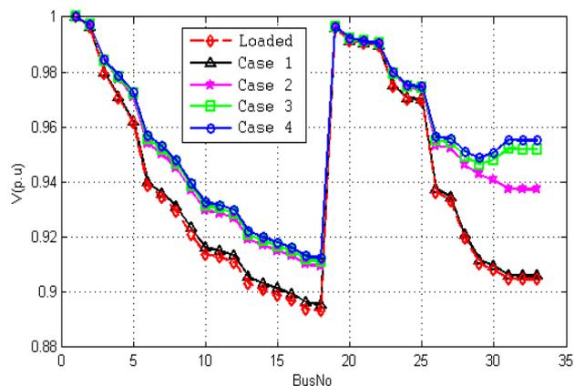
**Figure.5:** Voltage profile for various cases at type 2 load condition using proposed method
