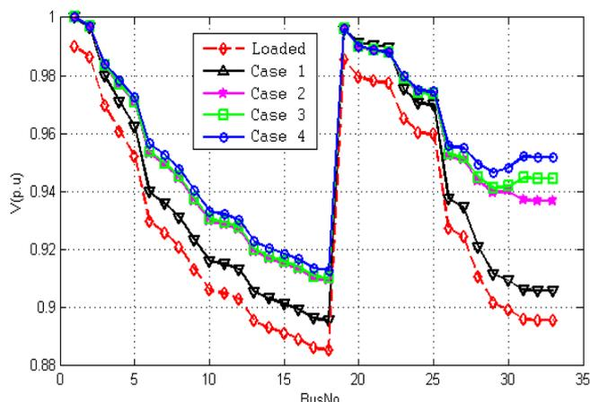
**Figure.6:** Voltage profile for various cases at type 3 load condition using proposed method
