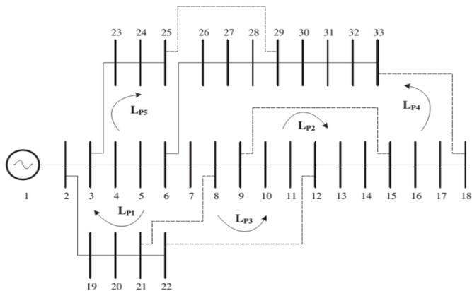
**Figure.3:** IEEE 33 bus radial distribution system single line diagram
