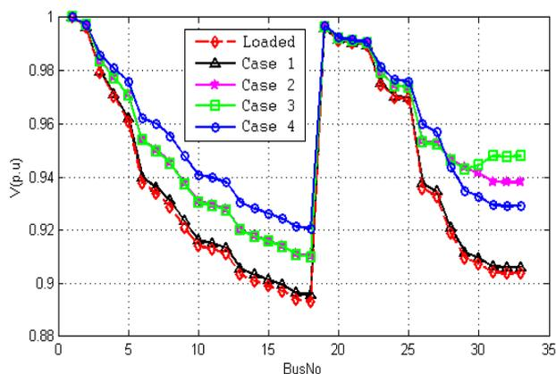
**Figure.4:** Voltage profile for various cases at type 1 load condition using proposed method
