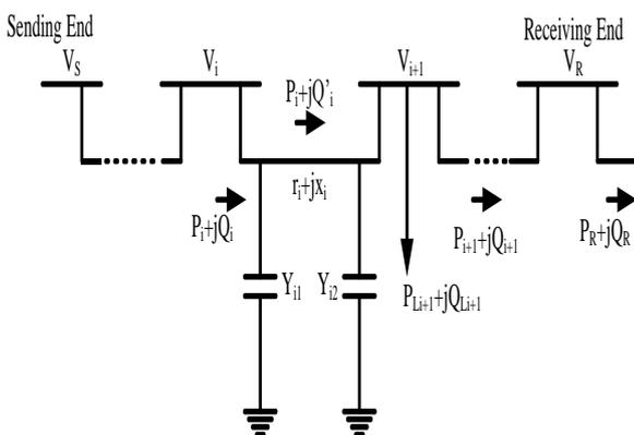
**Figure 1:** Line diagram of the distribution system
