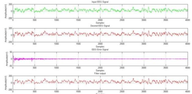
**Figure 3:** Output waveform for ALE – LMS EEG signal processing in MATLAB environment
