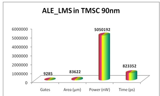
**Figure 7:** ALE – LMS utilization summary in TMSC 90nm
