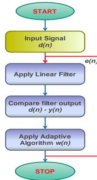
**Figure 2:** Flow diagram for ALE – LMS algorithm
