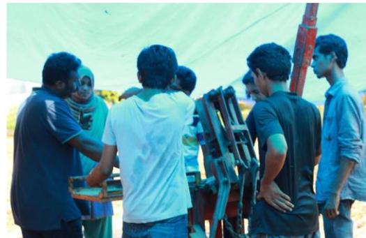
**Figure 2:** Production of CSEB blocks using the Auro 3000 from Auroville and the help of Architects in the region.
