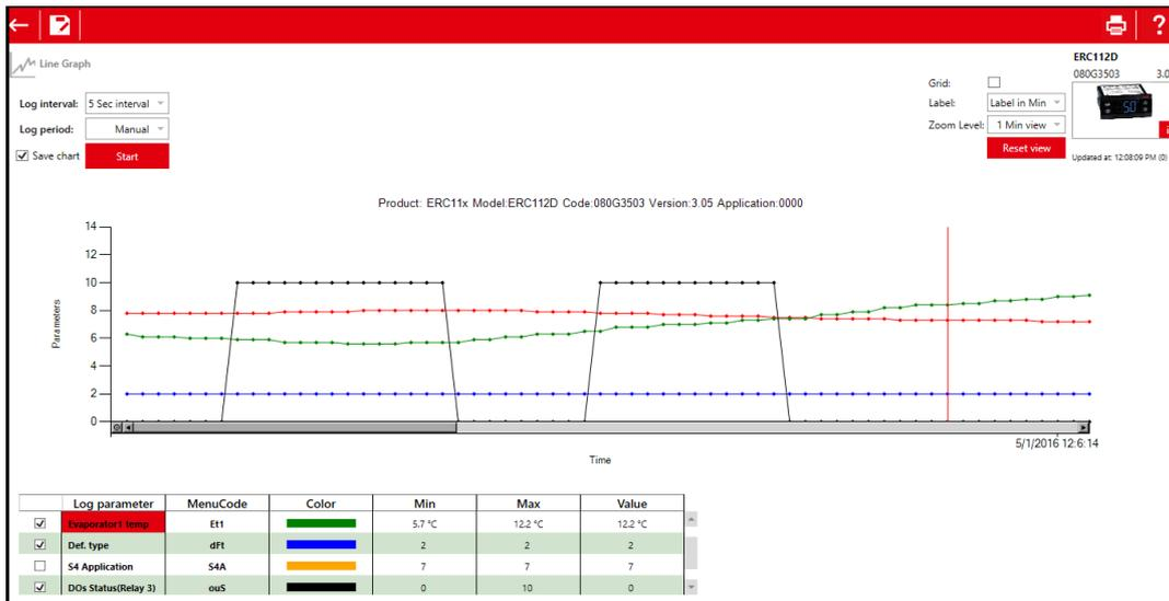
**Figure 4:** Monitoring parameters on Kool Prog PC tool
